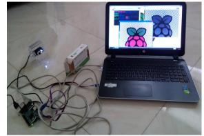
Fig. 4 Setup of Capturing an Image and Giving it in the form of RGB and Gray Format
